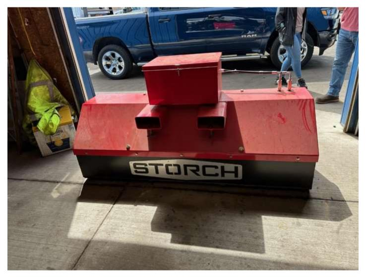
While in Michigan last summer I came across this innovative piece of equipment at a large selfservice facility. US Auto Sterling Heights found an incredible tool to magnetically sweep the grounds to pick up problematic debris. The magnet fits on the forks of the lift truck. They saw this unique tool being used by the city road maintenance department and added to their process.
